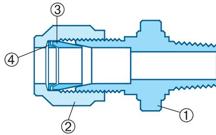
BULK compression fittings are made by four parts consisting of **body (1)**, **nut (2)**, **front ferrule (3)**, **back ferrule (4)**.
