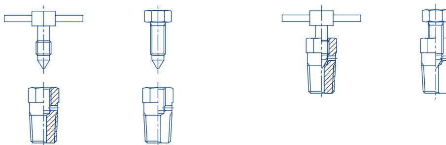
Condensing pots are used in steam metering lines to cool and condensate steam.
